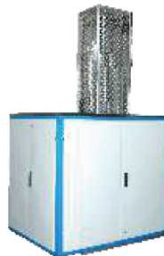
INSMART CIP installed at BARC, Mumbai Capacity: 100mm dia x 600mm height
